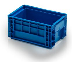
KLT crates with a smooth sub-floor and waterdrainage holes in the can ideally be used for areas where liquids shall be drained off. Stable impact surfaces on the front and the sides allow the use in mini-load system; lifting slots the vertical retrieval and special holes the fixing of lid sealings. Perfectly usable for manual handling due to their ergonomic grips at the front walls and their practical support grips on the side walls.
